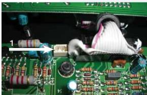
Closeups of the led PCB cable and connector are shown above. The black wire of the cable is closest to the ribbon cable. The cable only fits in one way.
